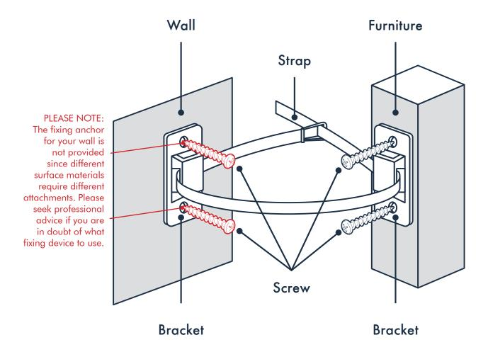
The safety hardware must be installed before use.
